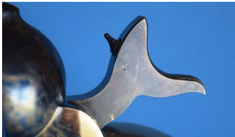
↑ Original features and details matter to enthusiasts. This Uberti has a proper hammer nose and no transfer bar.
