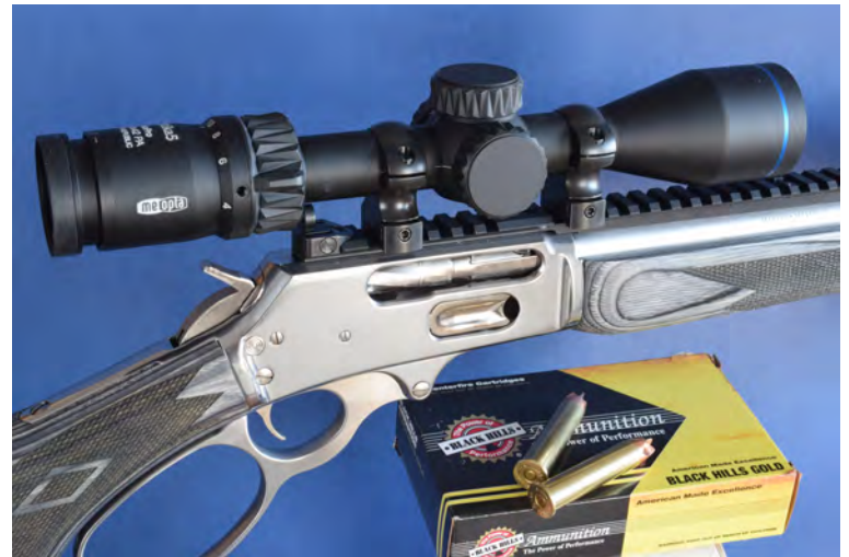
↑ The author installed a Meopta Optika 5 2-10x42 scope on the rail, without removing the ghost ring sight.
