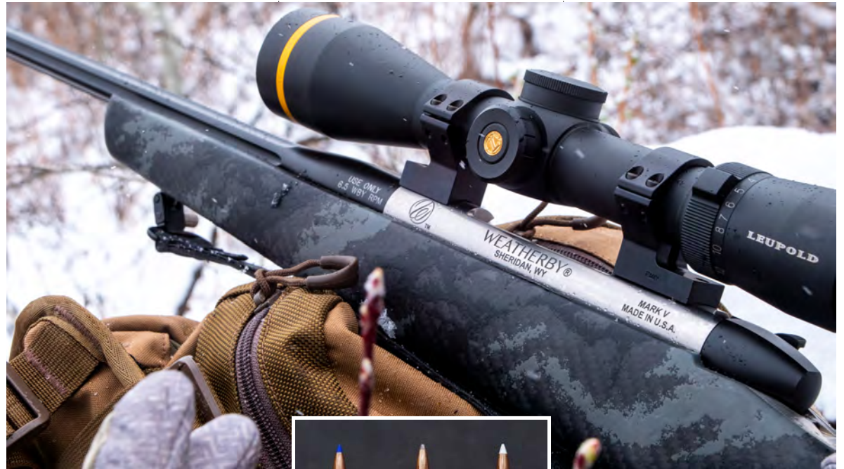
← The 6.5 WBY RPM was Weatherby’s first Rebated Precision Magnum round, created to maximize the potential of the company’s Mark V six-lug action. The new .338 WBY RPM uses the same smaller-diameter rim.
