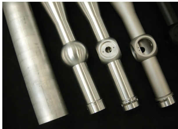
← CNC machining of scope tubes from thick-walled tubing ensures strength and holds tight tolerances.
