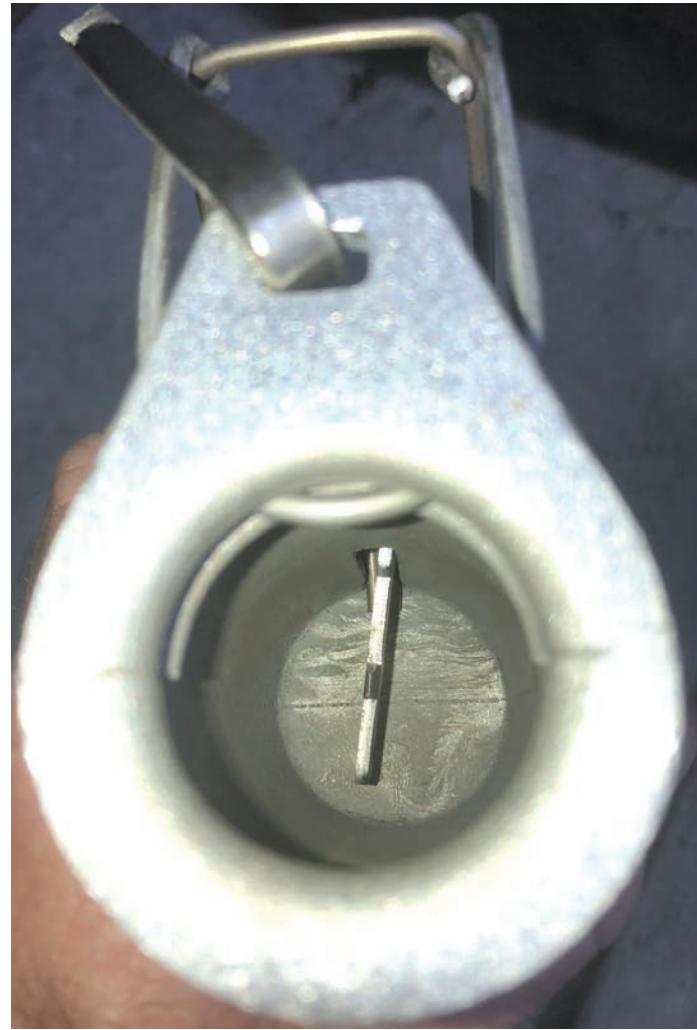
→ A raccoon reaches into this trap, tripping the trigger as it grasps the bait.
